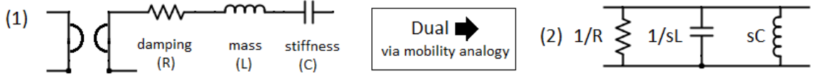
Figure 2.7: The corresponding circuits for Fig. 2.8 (1) and (2), before (1) and after (2) mobility networking. Due to the gyrator, the mechanical components becomes dual when they are seen on the electrical side of the network. As investigated in Fig. 2.8, this makes the shape of the Z_{mot} circle.
