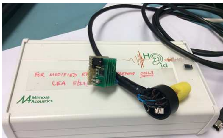
Figure 47: The purpose of this modification is to reduce crosstalk due to the long wire of ER10C probe. This reveals that small changes in the wire may lead significant property changes of the probe. The key idea is to amplify the microphone signal before it passes through the long wire. Near the probe's head we placed amplifier as shown in this picture.
