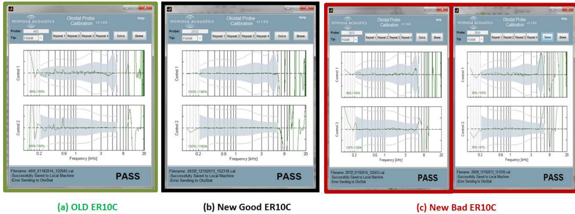
Figure 34: (a) Brass material for the middle tube holder part (the brass holder). RTV silicon is used to block the holder’s side hole. Calibration passes up to 9-10kHz (ER10C with 3 digits serial number) (b) Aluminum material for the chamber. RTV silicon is not used to block the holder’s side hole, but some of black material seals the side hole. Calibration passes up to 6kHz (ER10C with 4 digits serial number). (c) Aluminum chamber is used. None of material seals the holder’s side hole, a portion of the hole could be sealed randomly. Calibration totally fails or sometimes it passes but is unstable usually above 4kHz (ER10C with 4 digits serial number). Also (based on the manufacturer), the type of wire used in ER10C has been changed.
