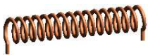
Figure 1.26: A solenoid is a uniform coil of wire. When a current is passed through the wire, a uniform magnetic field intensity \mathbf{H} is created. From a properties point of view, this coil is indistinguishable from a permanent bar magnet, having north and south poles. Depending on the direction of the current, one end of a finite solenoidal coil is the north pole of the magnet, and the other end is the south pole. The uniform field inside the coil is called solenoidal, a confusing synonym for irrotational. Figure taken from Wikipedia.
