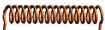
Figure 1.38: A solenoid is a uniform coil of wire. When a current is passed through the wire, a uniform magnetic field intensity \mathbf{H} is created. From a properties point of view, this coil is indistinguishable from a permanent bar magnet, having north and south poles. Depending on the direction of the current, one end of a finite solenoidal coil is the north pole of the magnet, and the other end is the south pole. The uniform field inside the coil is called solenoidal, a confusing synonym for irrotational. (Figure from Wikipedia.)
