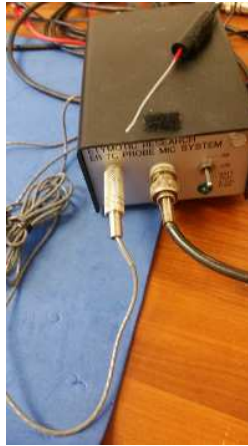
Figure 9: Etymotic Research 7C probe microphone.
