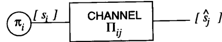
Fig. 2. The human acoustic channel is represented here as a hypothetical information-theoretic M -symbol noisy channel. Input speech sounds spoken by an average speaker are received (heard) by an average listener. An input set of spoken phones [s_i] , labeled by i , are spoken with probability \pi_i . Errors occur in transmission as described by a transition probability matrix \Pi having elements \Pi_{ij} . The set of received phones is [\hat{s}_j] , indexed by j .
