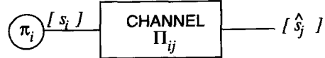
Fig. 2. The human acoustic channel is represented here as a hypothetical information-theoretic M -symbol noisy channel. Input speech sounds spoken by an average speaker are received (heard) by an average listener. An input set of spoken phones [s_i] , labeled by i , are spoken with probability \pi_i . Errors occur in transmission as described by a transition probability matrix \Pi having elements \Pi_{ij} . The set of received phones is [s_j] , indexed by j .
