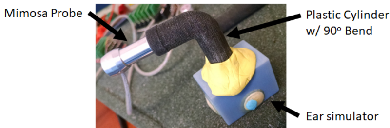
Figure 5.12: Measurement of a 90° bend in a uniform-area horn 7.5 [mm] in diameter.
