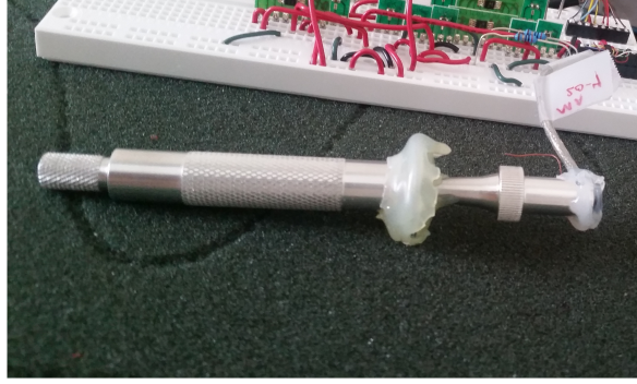
Figure 4.10: Probe tip connected to a uniform cylindrical syringe of 7.5 [mm] diameter. A jump discontinuity between the probe tip and the syringe was created using a washer as a flat plane, fused to the probe tip using a glue gun. To measure the two-port parameters of the probe tip, the plunger depth was varied (and carefully measured) to create test cavities of known impedance.
