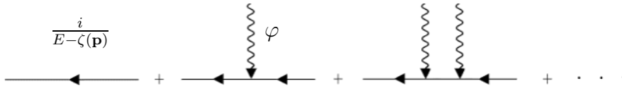
FIGURE 2.1 This diagram displays the piece of the collective action (2.12). The original fundamental particle (fat line) can enter and leave the diagrams only via external currents. It emits an arbitrary number of plasmons on its way (wiggly lines).
