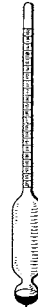
FIG. 171. The constant-weight hydrometer is a convenient instrument for finding the specific gravity of a liquid when precision is unnecessary.
