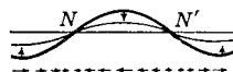
FIG. 214. Graphical representation of the displacements of the particles in a stationary longitudinal wave. The particles have just begun to return from their positions of maximum displacement, from the heavy to the light line. At the node N a condensation is forming, and at N' a rarefaction. After half a period conditions will be reversed. In the neighborhood of any given antinode, however, the particles are moving in the same direction with approximately the same speed, so that their relative positions are only slightly changed.
