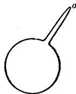
FIG. 112. Bulb for determining the density of a vapor by the method of DUMAS
