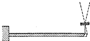
FIG. 100. Measuring the expansion of a bar with an optical lever
