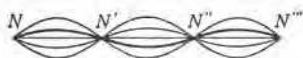
FIG. 213. Stationary transverse wave in a stretched string. The heavy line shows the position of the string at a given instant. When the segment NN' is moving up, that between N'N'' is moving down, and vice versa
