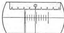
FIG. 267. Field of view of micrometer microscope
