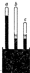
FIG. 124. In a the space above the mercury column contains nothing but mercury vapor. In b a small quantity of some volatile liquid has been introduced into this space. In c the volume occupied by the vapor has been decreased by lowering the tube, but the height of the column of mercury has remained unchanged
