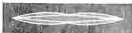
FIG. 238. Appearance of a string which is vibrating so as to produce its fundamental and first overtone simultaneously
