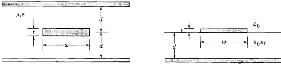
FIG. 8.6 (a) Stripline. (b) Microstrip.
