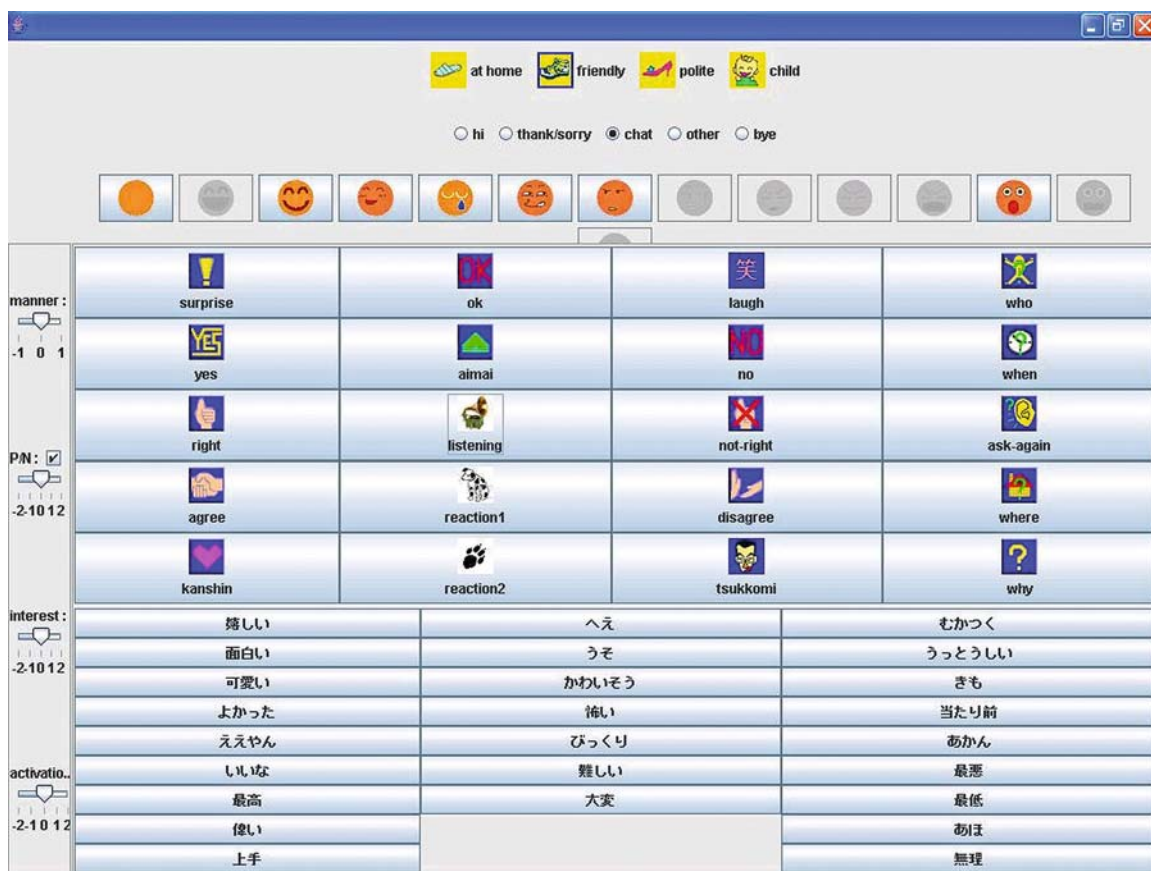
Fig. 25.4 The Chakai conversational speech synthesis interface. By clicking on a speech-act icon, a choice of emoticons is displayed in the upper section of the screen according to corpus availability, from which an utterance having the appropriate speech characteristics can be selected. Utterances are selected at random from among those in the same category within the corpus so that subsequent selection of the same combination will provide natural variety without unnecessary repetition
