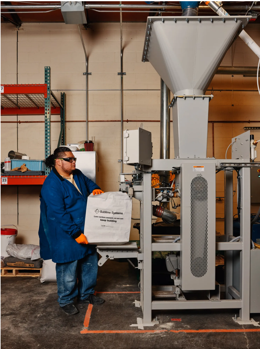
A Sublime employee sets up a cement bag, ready to fill it with the company's cement before shipping it out to customers.
